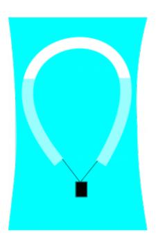
When the balloon is in the closed bottle, the pressure increases when the bottle is squeezed. The increase in pressure compresses the air bubble in the tube and the volume generating the buoyancy decreases - the balloon sinks. If, on the other hand, you reduce the pressure on the bottle, the pressure in the bottle decreases and the air bubble in the tube can expand - the buoyancy increases and the balloon rises.
